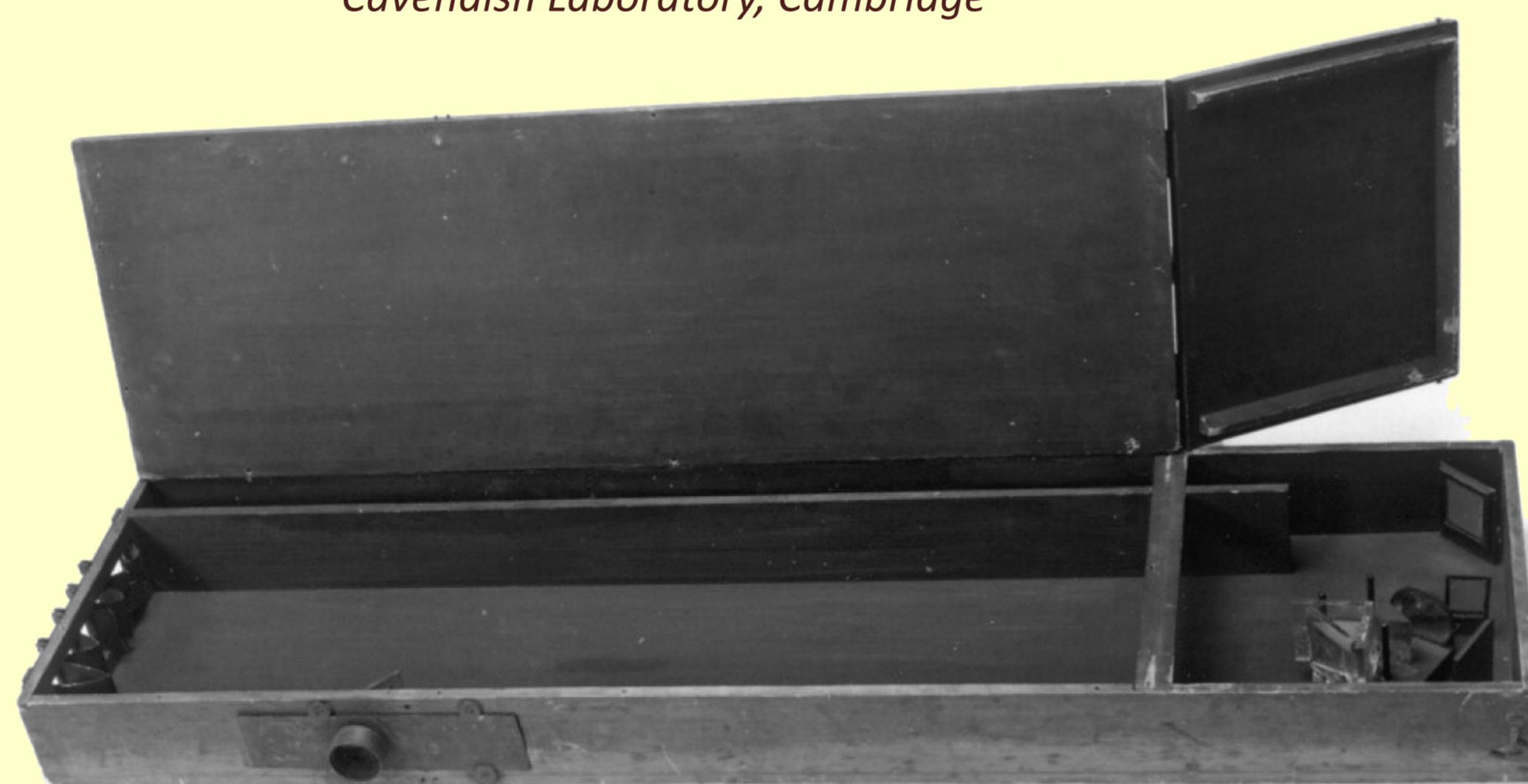
Maxwell's colour box , made by Smith & Ramage of Aberdeen, that he used to determine how spectral colours could be matched by 3 primaries. Courtesy Cavendish Laboratory, Cambridge
