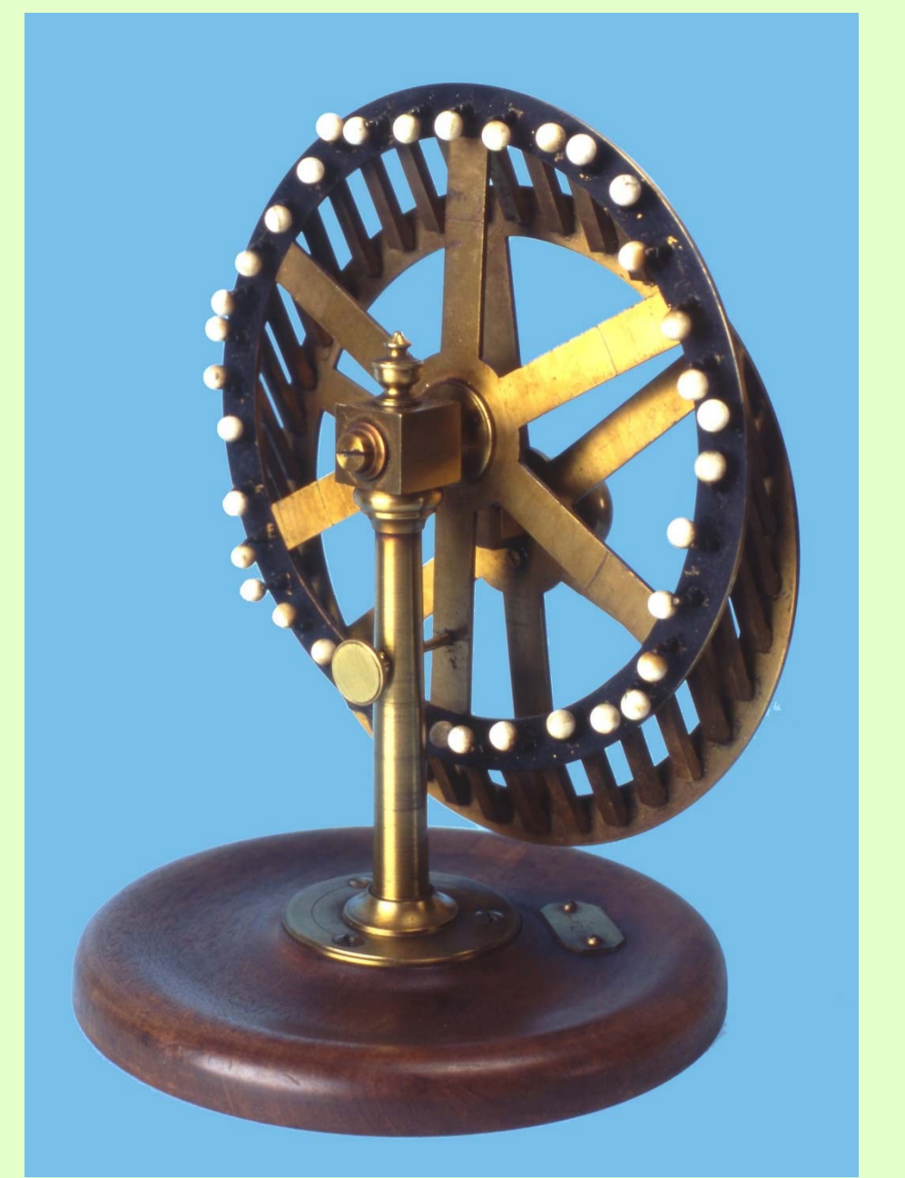
Model made in Aberdeen for Maxwell, illustrating his predicted wave motions on Saturn's rings
