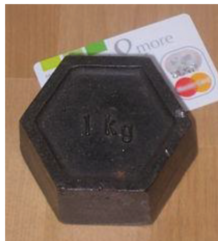
Domestic-quality 1 kilogram cast iron weight with credit card to show the scale. Courtesy of Martinvl via Wikimedia Commons.
