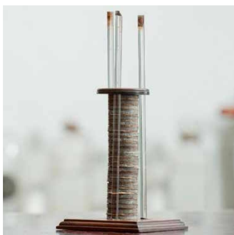
Figure 1: A voltaic pile made by Alessandro Volta and presented to Michael Faraday in 1814. Photo credit: the Royal Institution.
